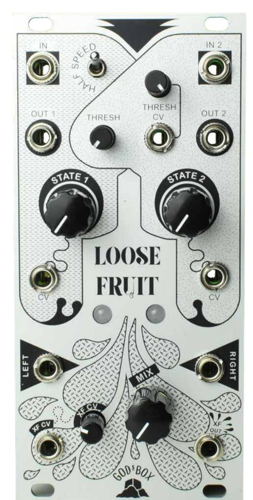
The Left waveshaper input is half normalled to the right: if nothing is plugged in to 'In 2', a signal plugged into 'In 1' will be connected to
